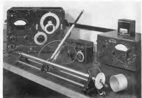
Figure 10. View of the component mount plugged into a General Radio slotted line for the measurement of a resistor.
