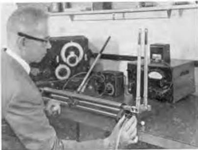
Figure 16. The Type 874-UB Balun in use with a slotted line to measure 300-ohm twin lead.
